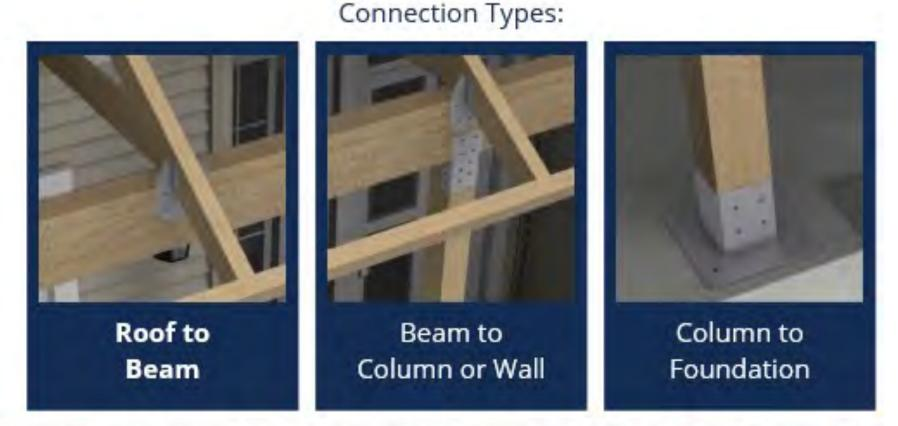
These connections allow the attached structure to resist the loads that try to tear it apart and minimize the chances that they will become flying debris
